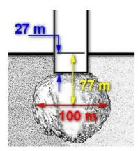
Position of a nuclear demolition charge in the above picture is exactly in the middle of a cavity.
